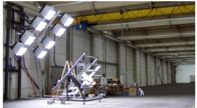
Fig. 3. Solar load testing apparatus in a laboratory that induces stresses similar to real application with the full UV, visible and infrared spectrum
